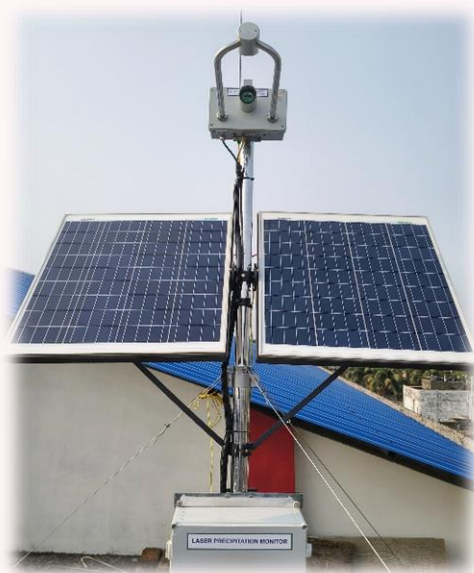
LASER Precipitation Monitor installed in college by NE Space Application Centre, (ISRO), Department of Space, Govt. of India.
